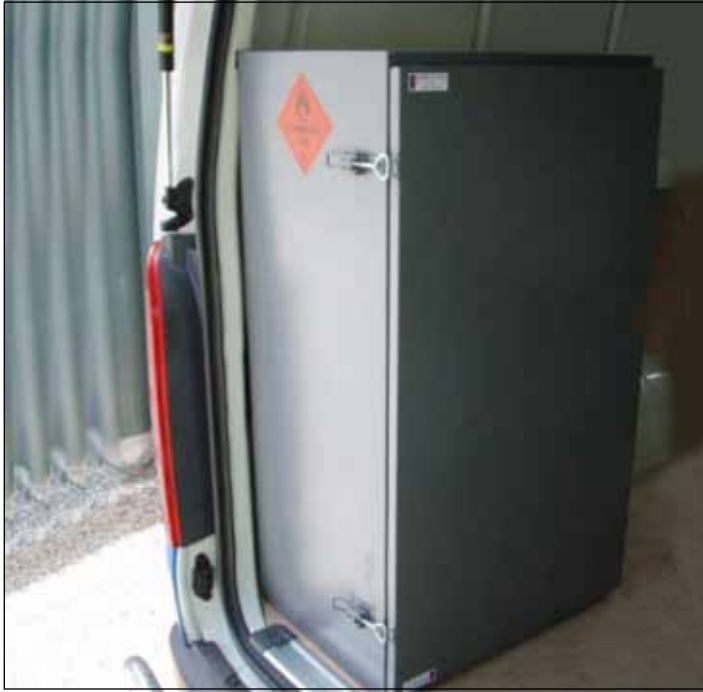
Figure 1: Ensure the gas cabinet is securely mounted, with vapour-tight seals on the door and around the vent pipe.
