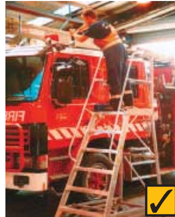
6.0 Use of mobile work platform to undertake maintenance.
