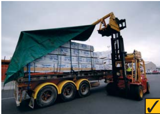
1.0 Tarping from the ground using a 'Barney Beam'.
